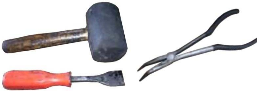
Figure 12 Typical Tools for Replacing Isolator Pads
