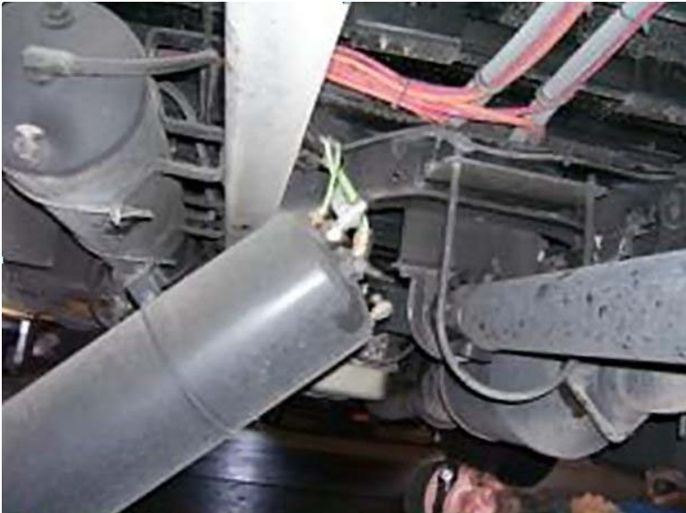
Figure 6 Air Tank Repositioned
