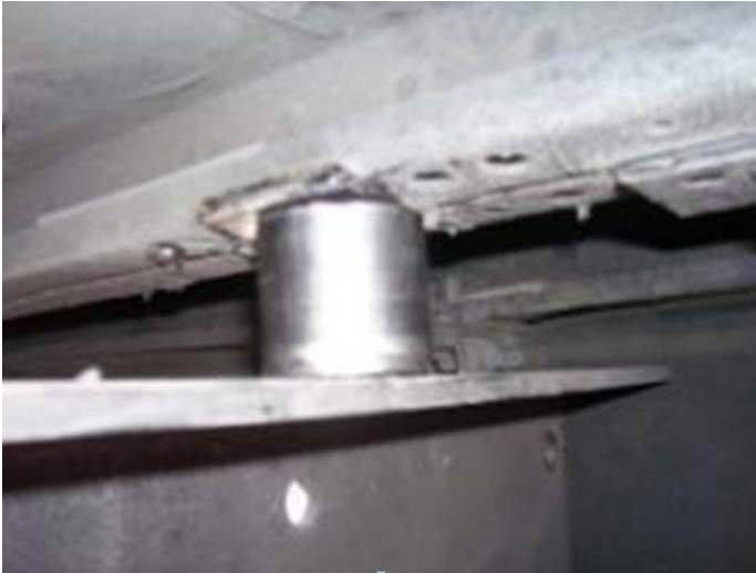
Figure 11 Use a suitable block to support the bus body while replacing the isolators
